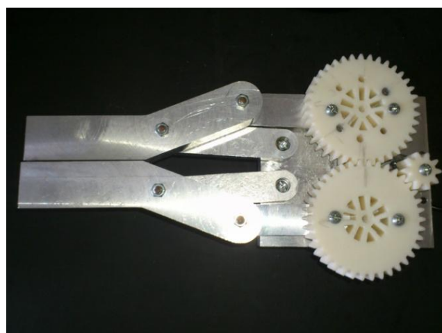
Figure 4.8 : The real automated gripper
