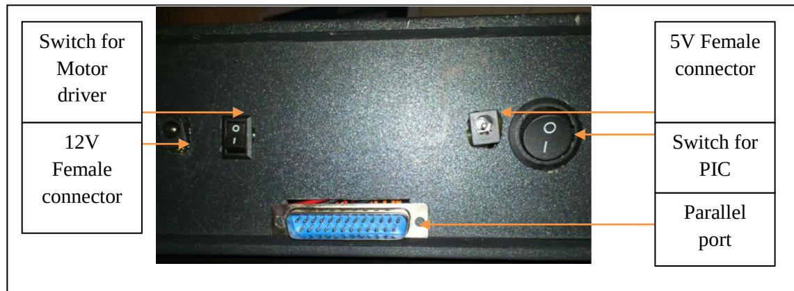
Figure 4.15 : The connector on the project box
