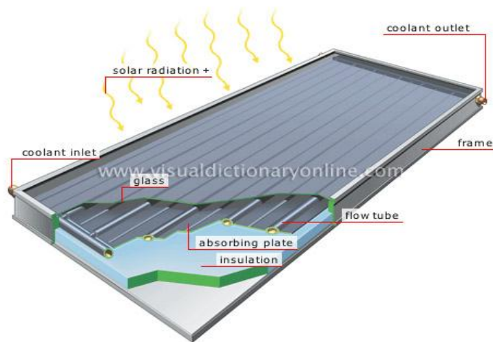
Figure 2.1: Flat-plate collector
