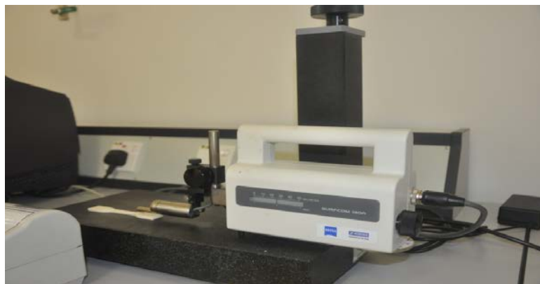
Figure 4.6: Surfcom 130A used to measure surface
