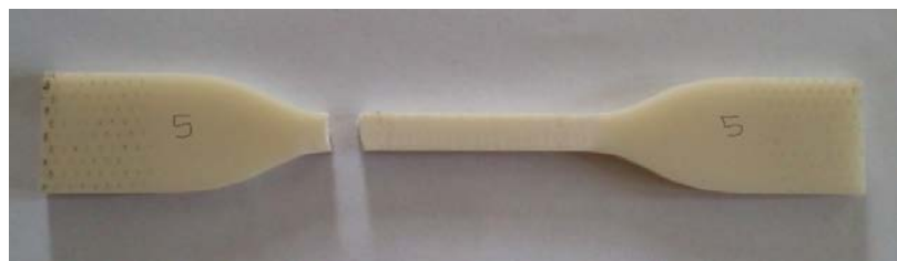
Figure 4.4: Specimen after fracture.
