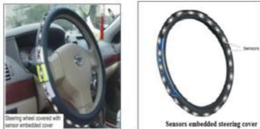
Figure 2.11: Sensor embedded steering wheel (Sources: Betsy Thomas Electronics et al, April 2008)
