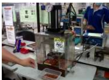
Stripping the aircoil
