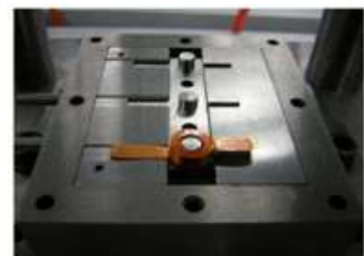
Trimming punch step down and cut the lead aircoil
