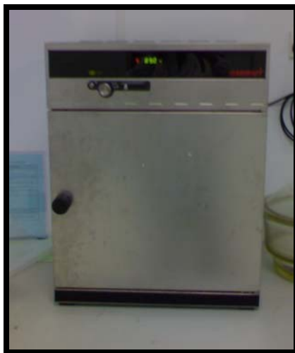
Appendix B1: Oven for drying OPF chips
