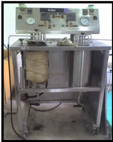
Figure 3.3.2 (a): M.K Digester
