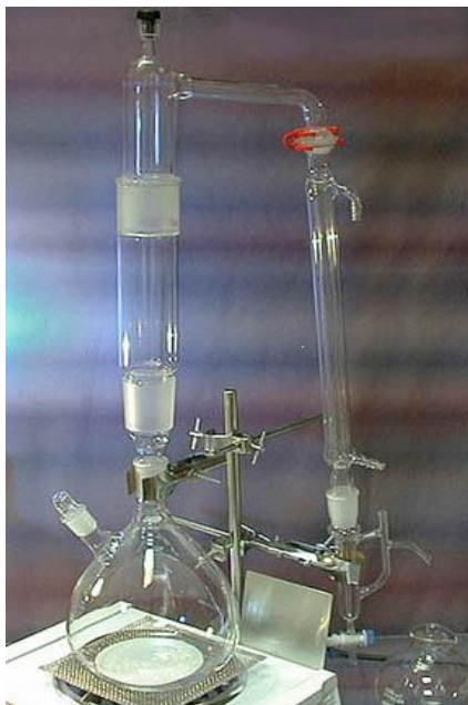
Figure 2.8 Lab-scale water distillation apparatus for essential oil extraction (Source: http://www.aromatherapy-essential-oils.org )
