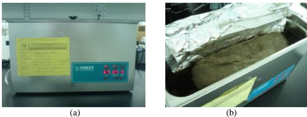
Figure 3.4 The ultrasonic pretreatment process (a) ultrasonic bath equipment (b) the gaharu sample inside loose cloth during pretreatment process
