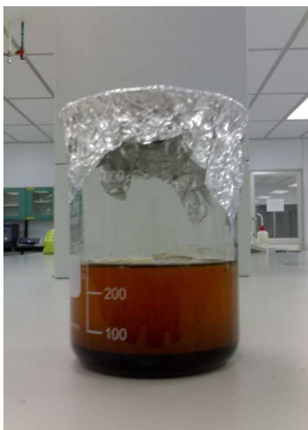
Figure 3.4: Layers formed after an overnight gravity settling
