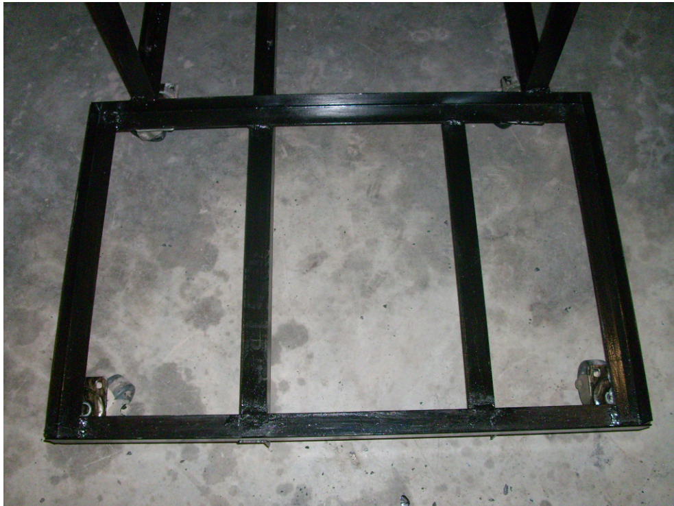
Figure 4.1.2: Hydraulic tank basement
