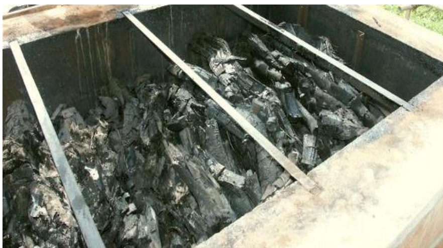
Figure A2: Making charcoal from retort
