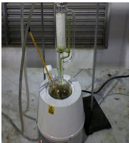
Figure 3.10: Soxhlet extraction process
