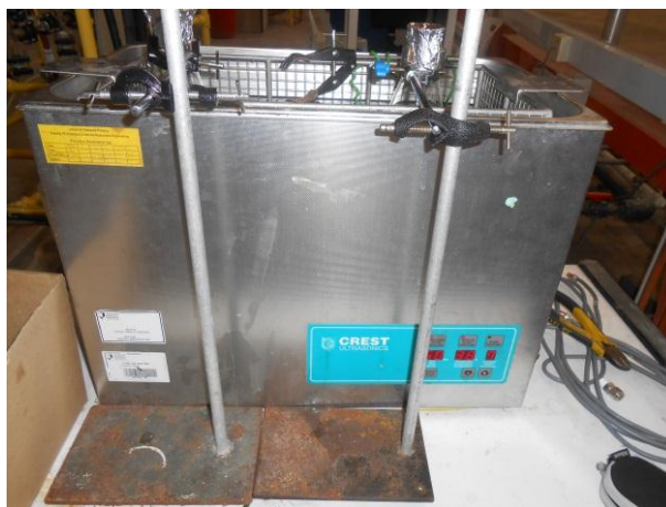
Figure 3.5 Ultrasonic extractor (Brand: CREST)
