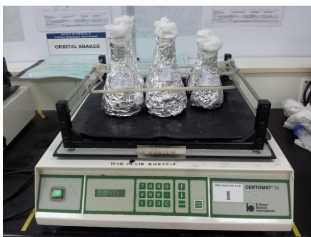
Figure 3.3 Orbital shaker (Brand: CERTOMAT SII )
