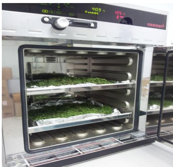
Figure 3.2 Drying oven (Brand: Memmert)
