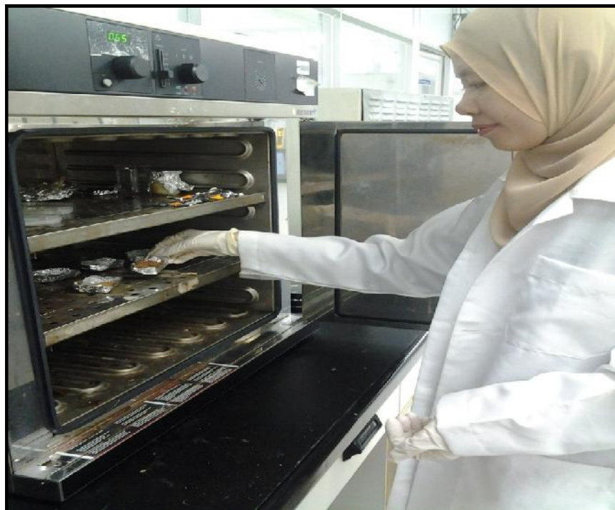
Figure 3.12 The sawdust in the oven for drying process at 60 °C
