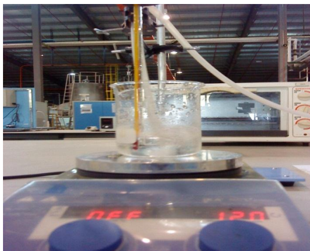
Figure A-2 CO 2 purged into DEA aqueous solution at constant stirrer speed, 120 rpm
