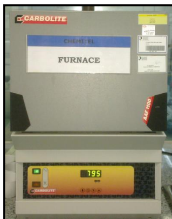
Figure B-1.5: The dried solid was calcined at 800 °C for 6 hr.
