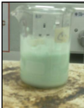
Figure B-2.6: Second wet co-impregnation was carried out at room temperature for 3hr.
