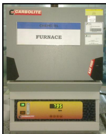
Figure B-2.8: The dried solid was calcined at 800 °C for 6 hr.
