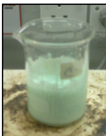
Figure B-2.3: First wet co-impregnation was carried out at room temperature for 3hr.
