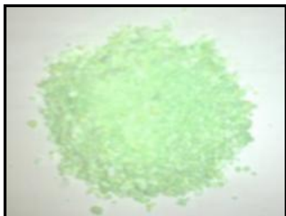
Figure B-2.4: Dried solid after first wet co-impregnation.
