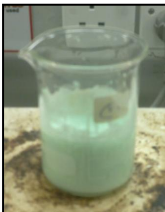
Figure B-1.3: Wet co-impregnation was carried out at room temperature for 3hr.
