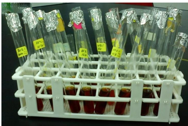
Figure 3.5 DNS method for determination of glucose concentration.
