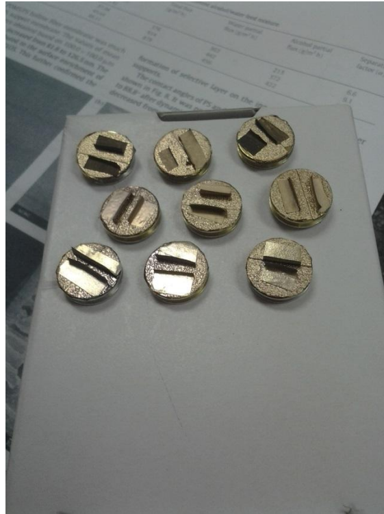
Figure A.7 Samples Coated With Layer of Gold For SEM
