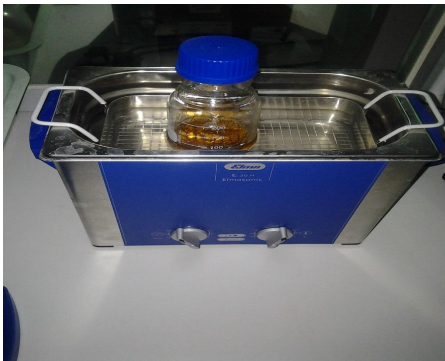
Figure A.3 Removing Bubbles In Ultrasonic Water bath
