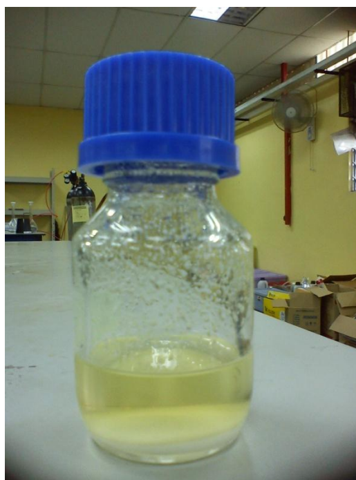
Appendix A.2.10: Mixing drying agent with biodiesel
