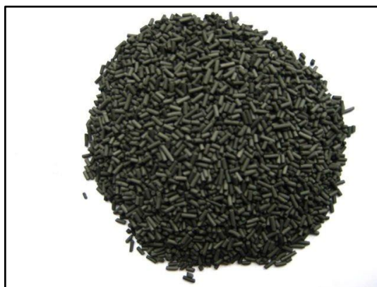
Figure 2.3 Activated carbon as solid sorbent in water purification method
