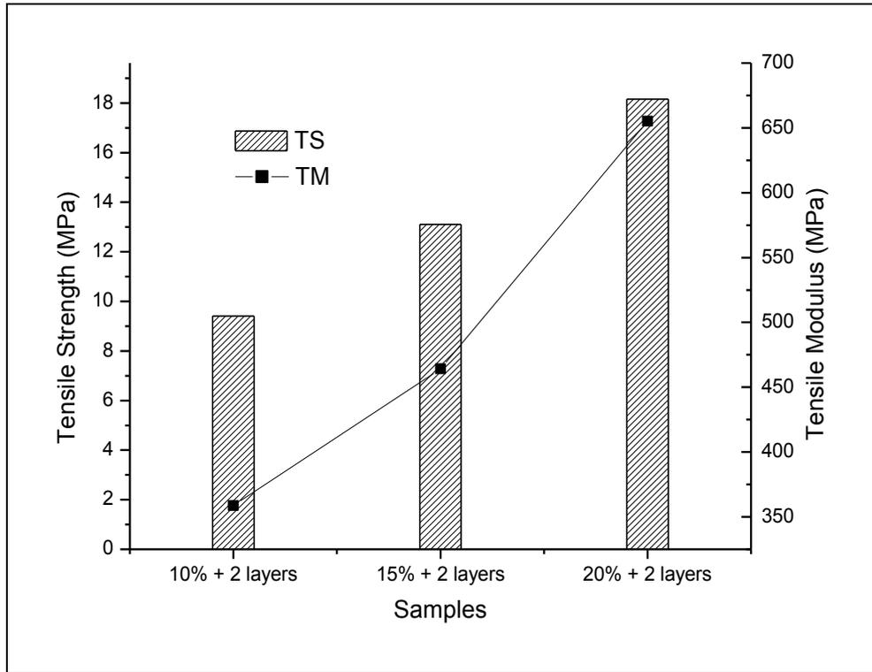
**Figure 4.3:** TS and TM of 2 Layers Composites with Various RCA Percentages
