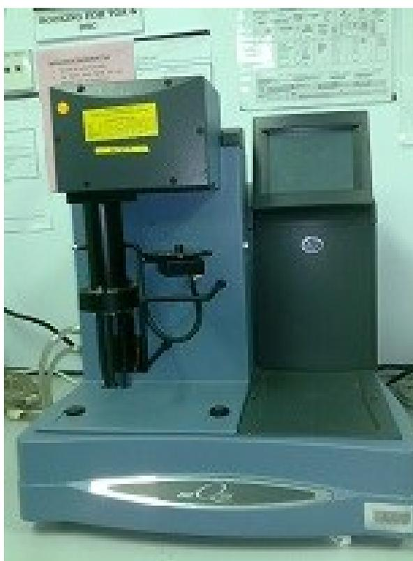
**Figure 3.9:** Thermogravimetric Analyser (TA Instrument, TGA Q500)
