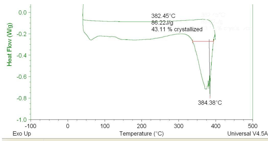
**Figure 4.2:** Various Thermal Properties of Pure Polyester
