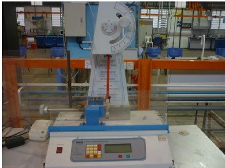
**Figure 3.7:** Impact Pendulum Tester (Model- ZWICK/ROELL)
