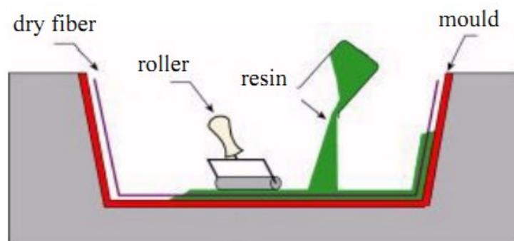
**Figure 2.4:** Hand Lay-up Method
