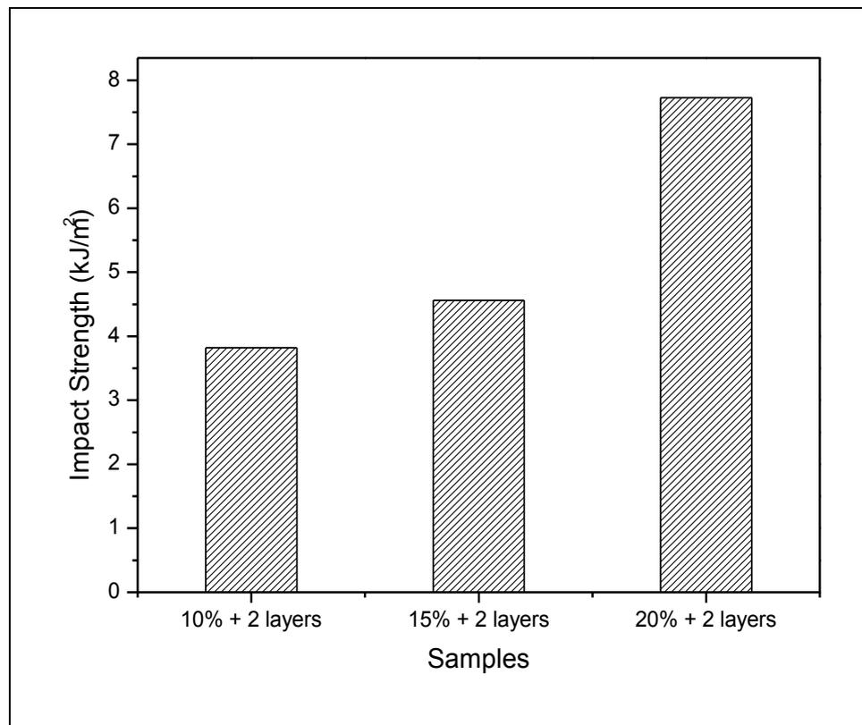
**Figure 4.4:** Impact Strength of 2 Layers Composites with Various RCA Percentages
