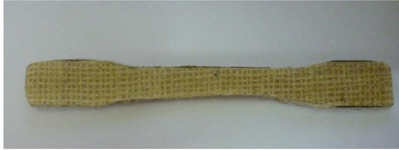
**Figure 3.6:** Composite Specimen for Tensile Testing
