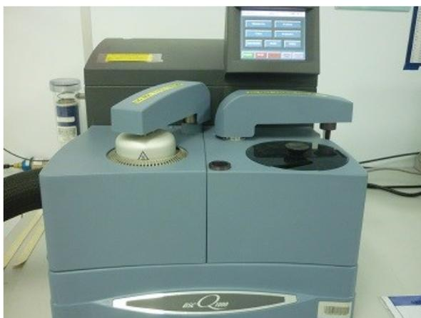
**Figure 3.10:** TA instrument, Q-1000 (DSC Analysis)
