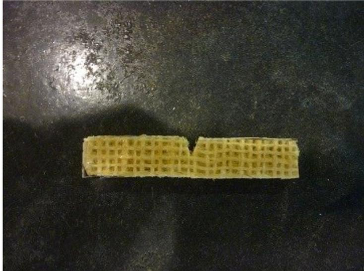
**Figure 3.8:** Notched Specimen for Charpy Impact Test
