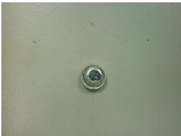
**Figure 3.11:** Aluminium Lid and Pan with Samples Inside
