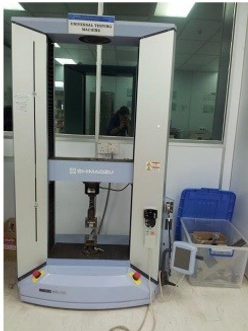
**Figure 3.5:** Universal Testing Machine AG-1 (Tensile Test)
