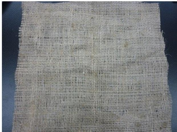
**Figure 3.2:** Kenaf Fibre Mat
