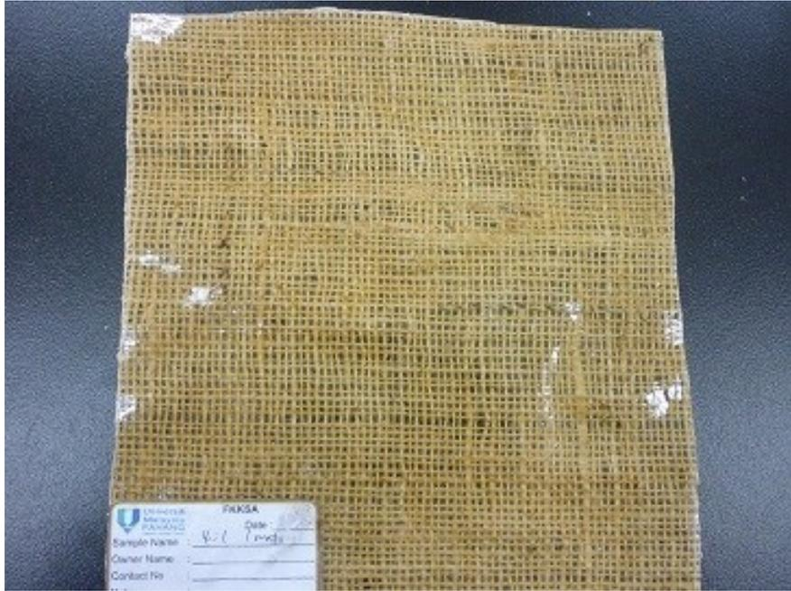
**Figure 3.4:** KPC with 20% RCA and 1 Fibre Layer
