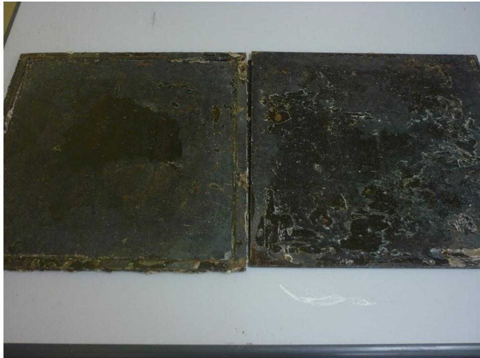
**Figure 3.3:** Hand Lay-up Method Mould
