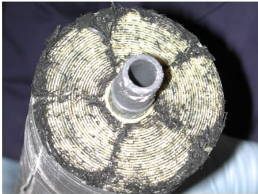
Figure A.1 Membrane Fouling
