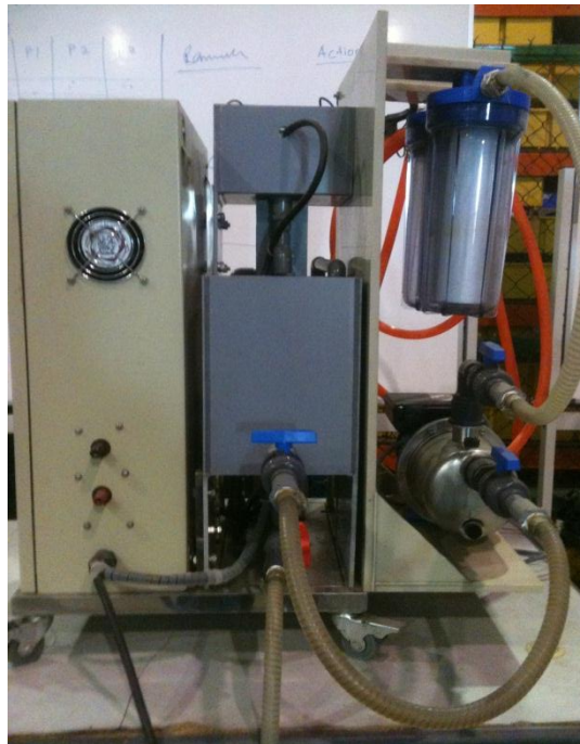
Figure 3.2: Electrocoagulation OT-1 (front view)
