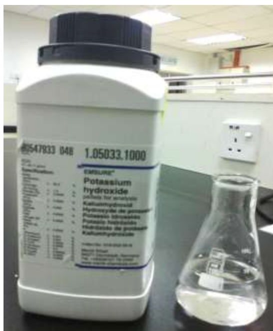
Appendix A.2.2: Mixing of alcohol and catalyst to produce methoxide
