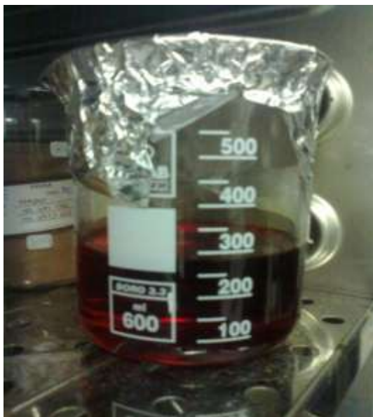
Appendix A.2.7: Biodiesel drying to remove excess water
