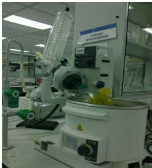
Appendix A.2.5: Water bath rotary evaporator
