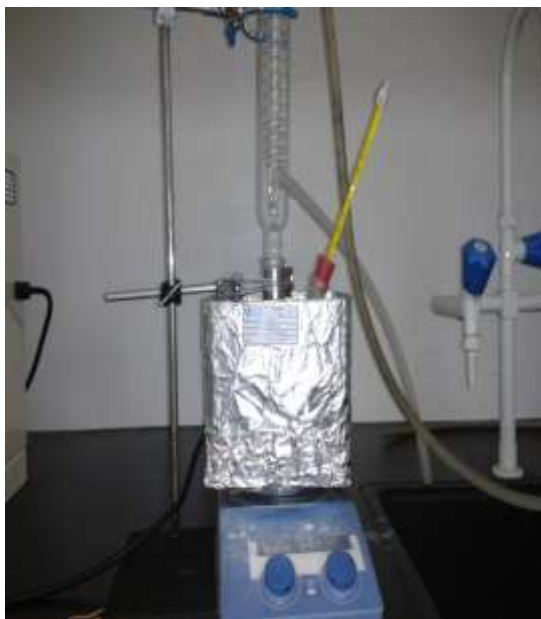
Appendix A.2.3: Mixing of methoxide and palm oil using reflux condenser
