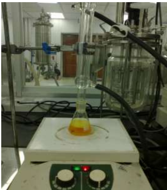
Appendix A.3.3: Heating of palm BD for saponification
