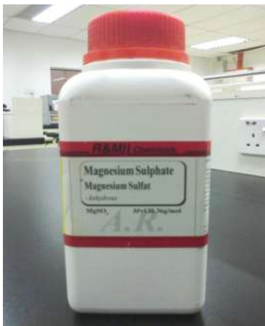
Appendix A.2.1: Addition of drying agent to remove excess water and impurities
