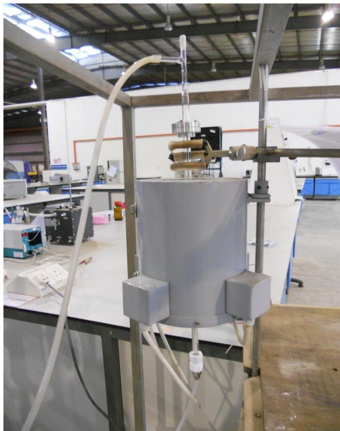
Figure 3.8: Tubular furnace with reactor
