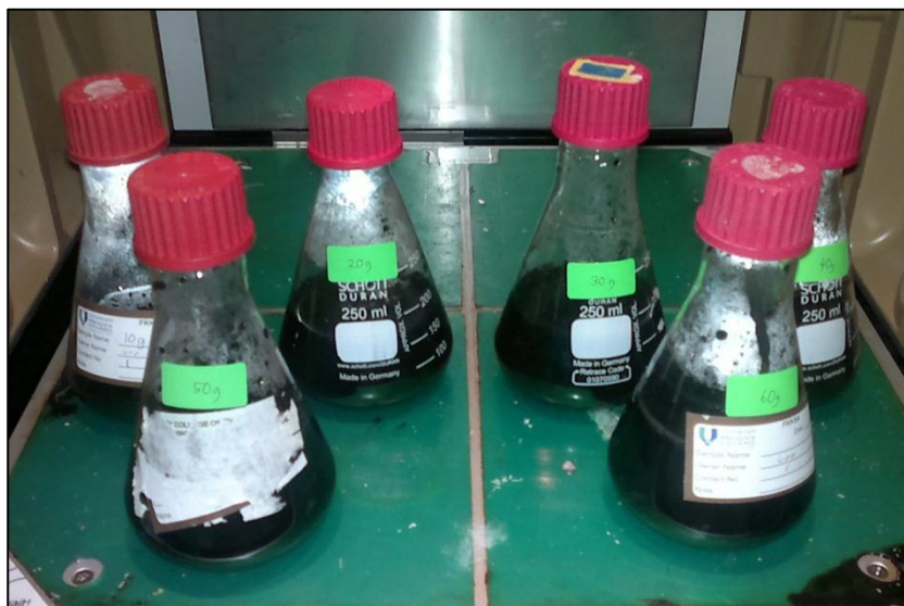
Figure B.2: Mixed solution with different amount of GAC is in the stackable incubator shaker
