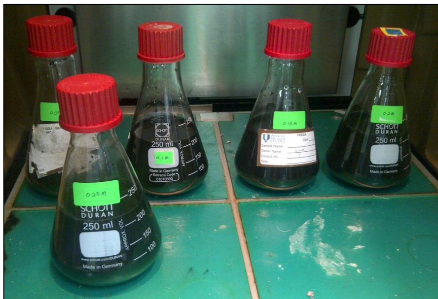
Figure C.3: After mixing the GAC and SBD, the solution is put into stackable incubator shaker
