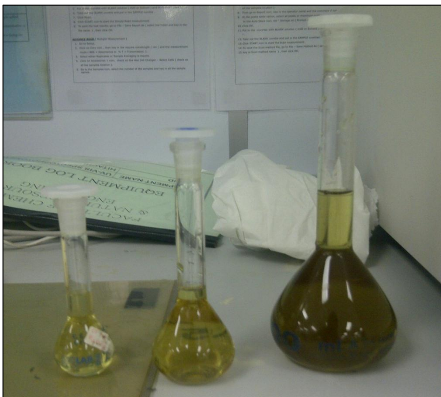
Figure 4.2: The solution with different volume and concentration for standard curve analysis (10 ml, 25ml, and 100 ml)
