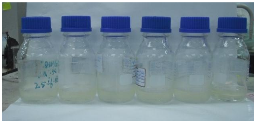
Figure D.6 Different agitation speed. From left is 50 rpm, 100 rpm, 150 rpm, 200 rpm, 250 rpm, and 300 rpm
