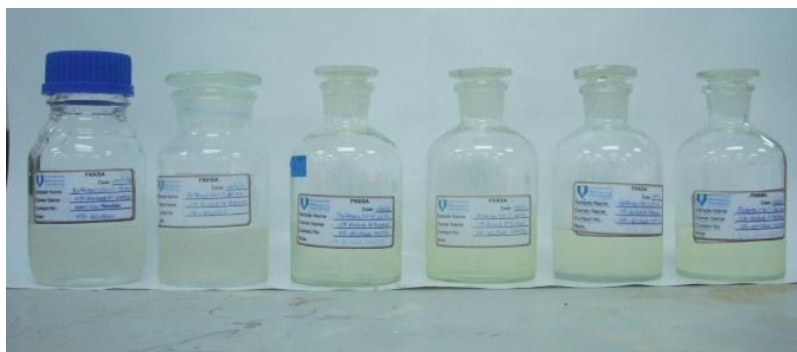
Figure B.6 Different extraction time. From left 15 minutes, 30 minutes, 60 minutes, 120 minutes, 180 minutes and 240 minutes
