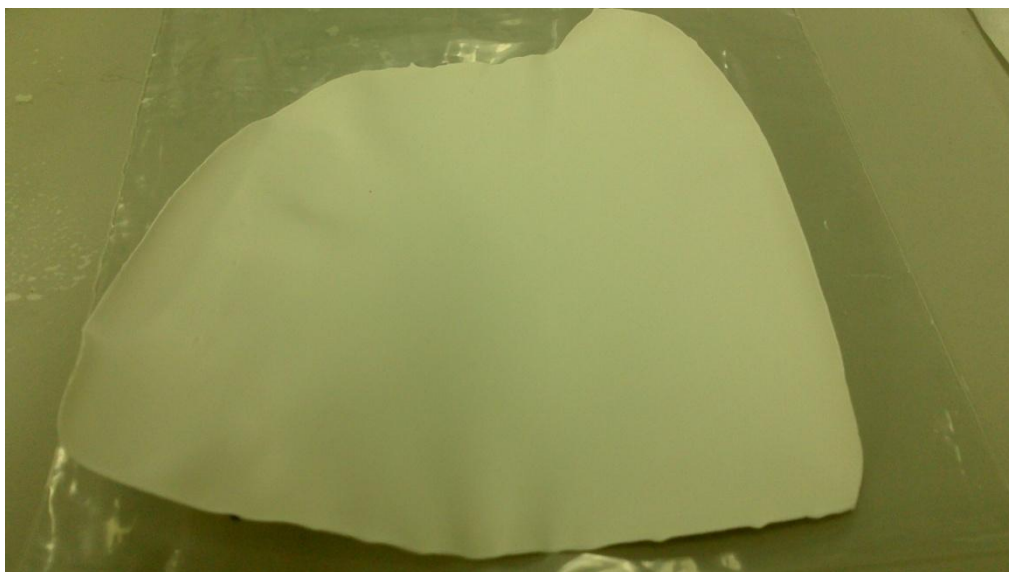
Figure 3.2 Flat sheet membrane after freeze dried.
