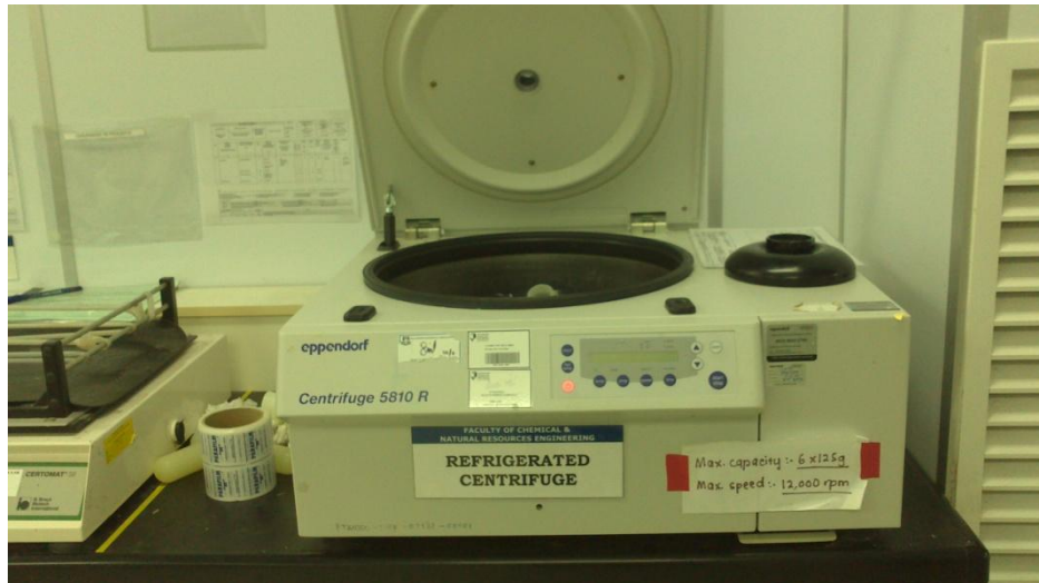
Figure A.5 Centrifuge 5810 R used to separate the ground resin from the copper ion solution.
