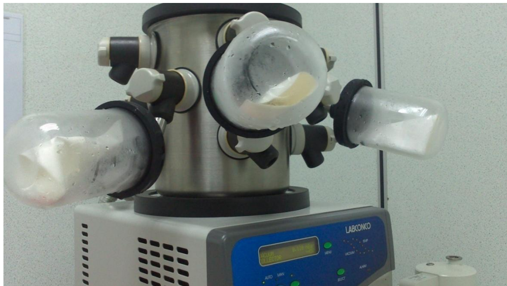
Figure A.4 freeze dryer used to dry the flat sheet MMM.
