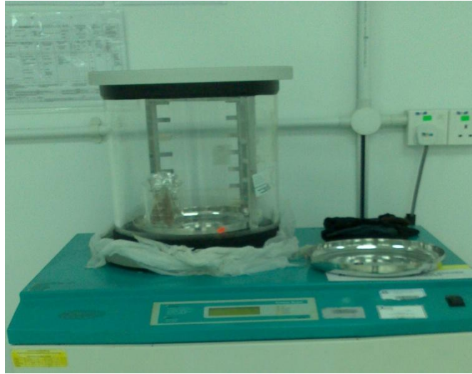
Figure A.1 Freeze dryer used to dry the resins.
