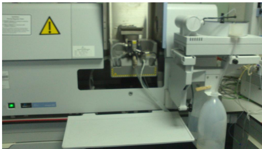
Figure A.6 Atomic Absorption Spectrophotometer used to measure heavy metal concentration.
