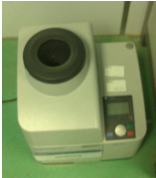
Figure A.2 Ultra centrifugal grinder used to grind the resins.
