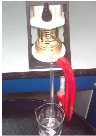
Figure A.7 Amicon stirred cell used in water flux experiment.
