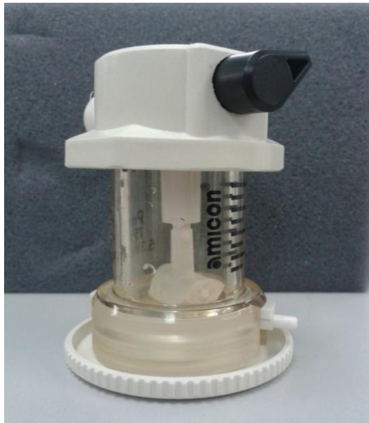
Figure 3.3 Amicon Stirred Cell model 8010 for measuring water flux.
