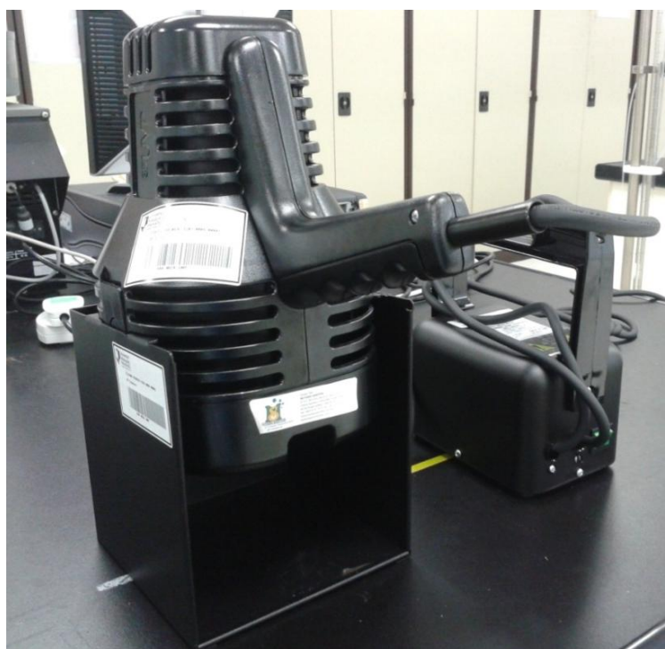
Figure 3.1 UV-Light Cell, Wave Length 365 nm (B-100AP Lamp. Brand: Ultraviolet Product (RDU100111) with Exposure Box for B-100 AP.
