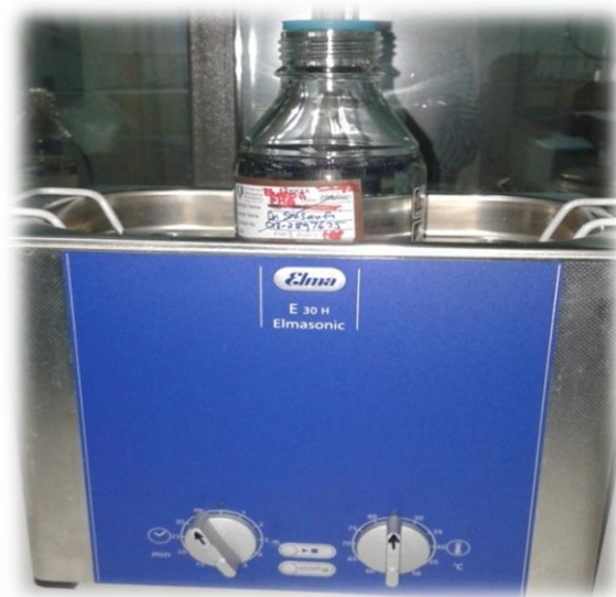
Figure A-2: The unmodified PES membrane was soaking within the ultrasonic.
