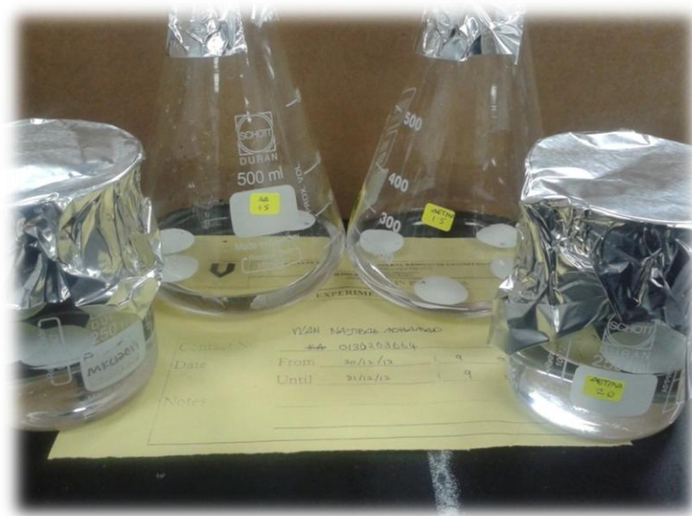
Figure A-3: The unmodified membrane was immersed into the monomer for 12 hours.
