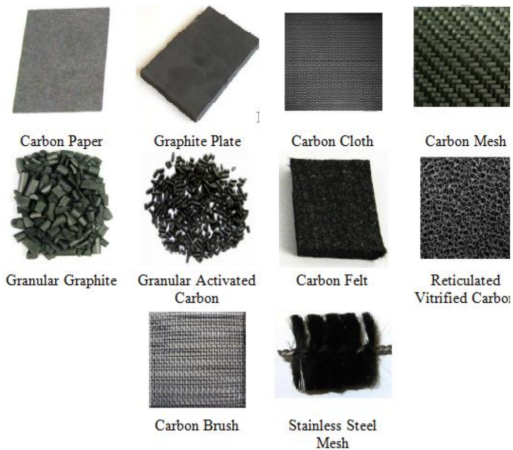
Figure 2.2 Electrode Materials Used for MFC
