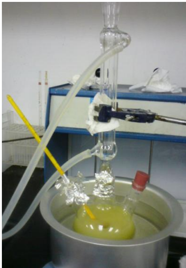
Figure 3.1 Experimental setup: 3 necked-flask equipped with condenser
