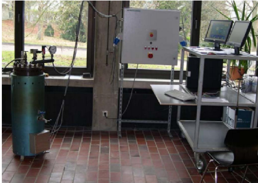
Figure 2.3 Equipment Used for Hydrothermal Carbonization Process (Remke et al ,200)
