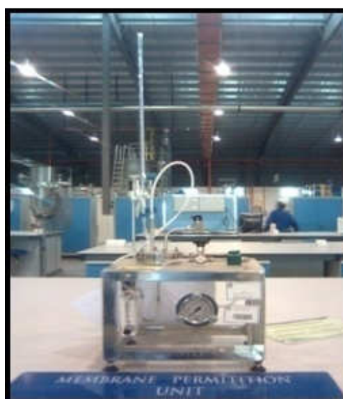
Figure 3.4: Photo of permeation unit use in this experimen
