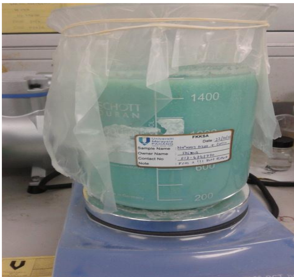
Figure 3.4: Modification of Na + MMT with CuCl 2
