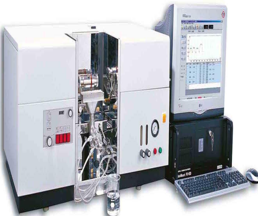
Figure 3.7: AAS Equipment (AAS 7003M)
