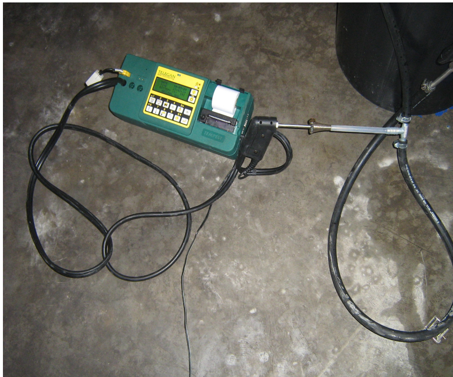
Figure 3.1 Analyze Acid Gas Content Using Gas Analyzer
