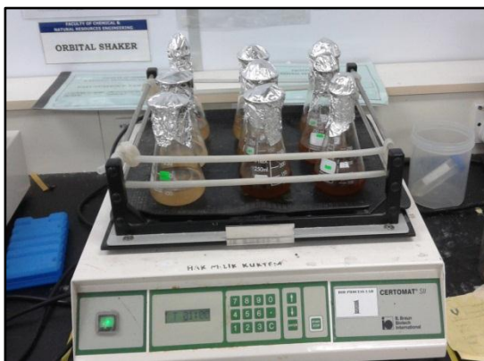
Appendix A7: Sample shaken on rotary shaker. Appendix A8: Sample after shaken.
