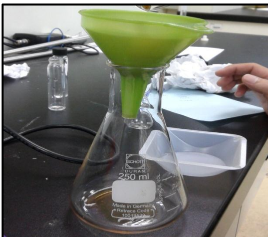
Appendix A11: Filter the sample before analyse using AAS.
