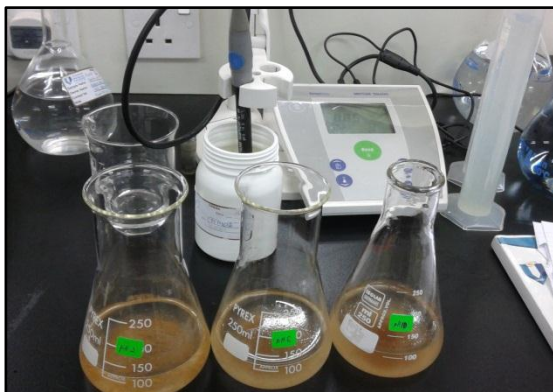
Appendix A5: Adjusting the pH of sample. Appendix A6: Sample before shaking on rotary shaker.
