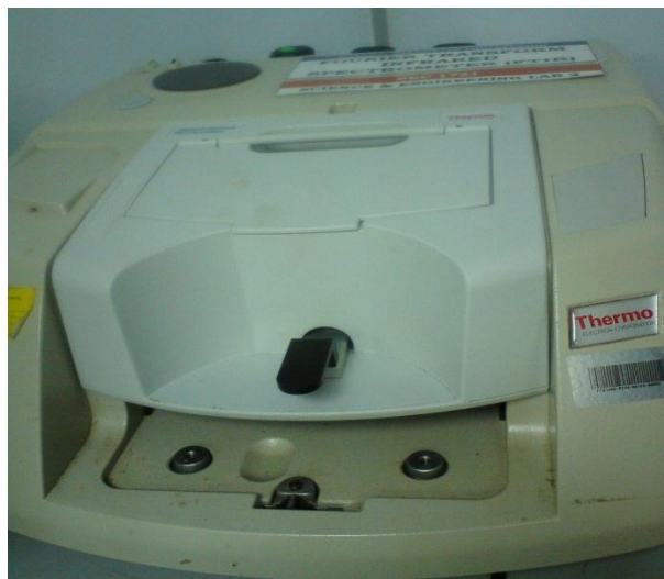
Figure 3.6 FTIR for powder sample
