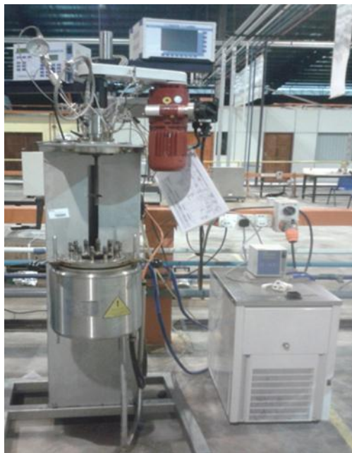
Figure 3.1 Supercritical unit Buchiglauster model
