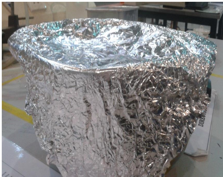
Figure 3.2 Clay bowl filled with WFW covered with aluminium foil
