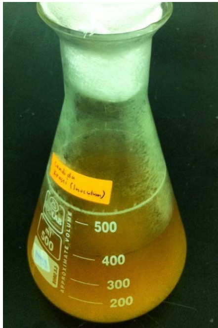
Figure 4.1 A. Growth medium (20g/L of glucose and 10g/L of yeast extract) after autoclave. B. Growth medium after cultivation for 24 hours at 36 °C with 180 rpm agitation speed.
