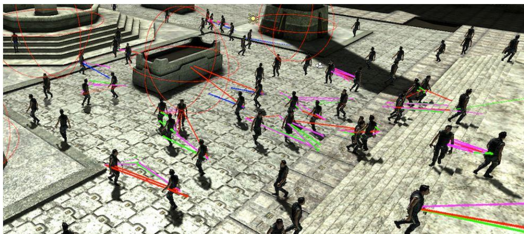
Figure 2.2: UnitySteer update to spherical obstacles avoidance
