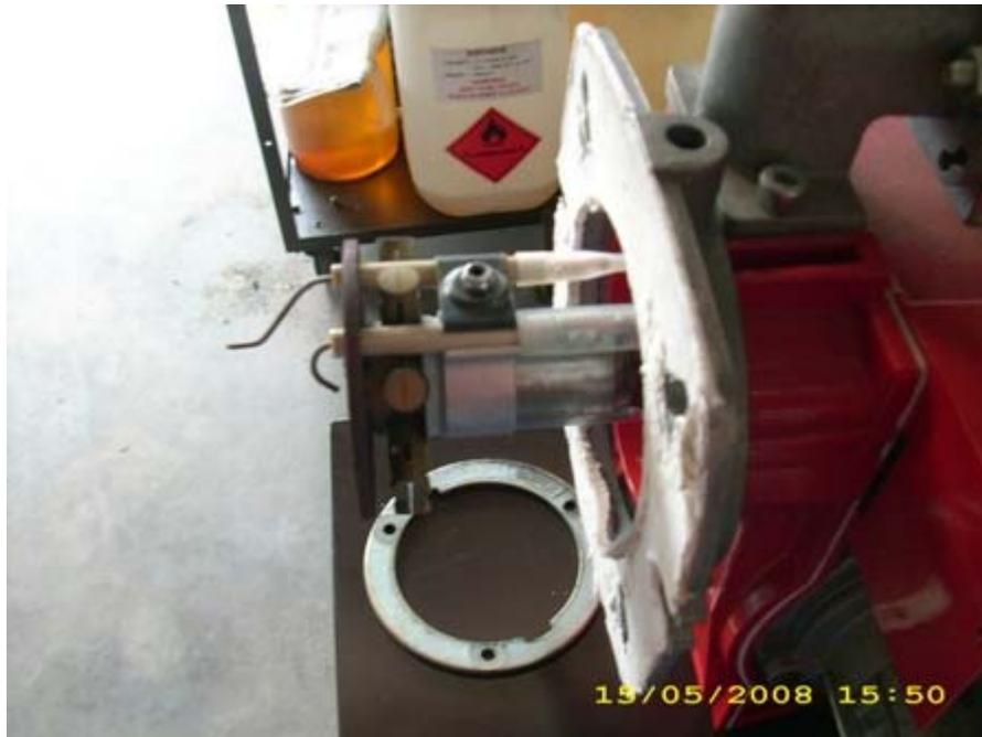
Figure 3.4: Picture of nozzle and air outlet
