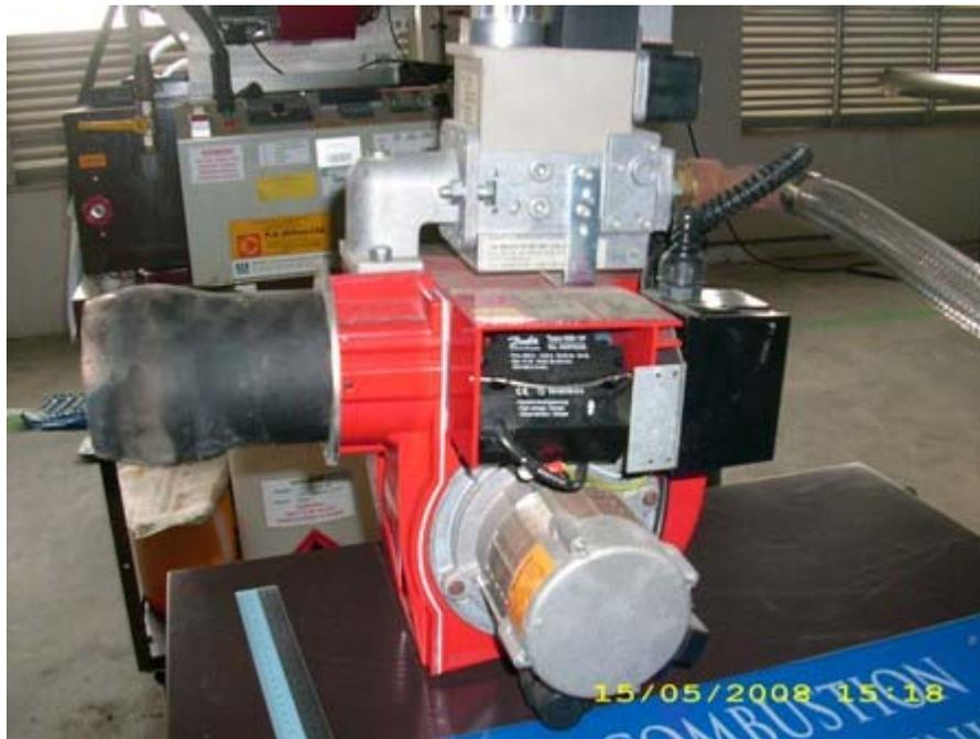
Figure 3.3: Picture of C492 Gas Burner
