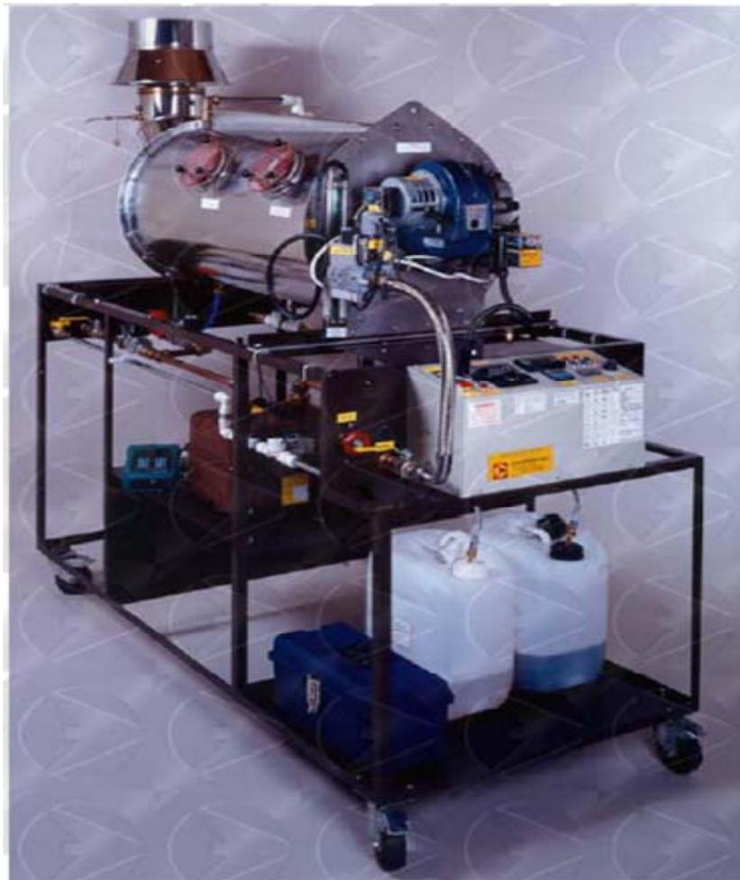
Figure 3.2: Picture of combustion laboratory unit C492
