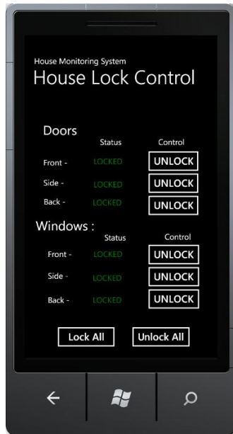
Figure 2.4.5: Access to House Lock Control interface in windows phone simulator
