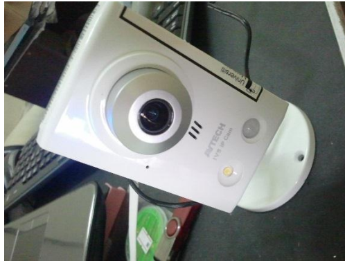
Figure 2.3.7.1.8: The IP Camera that have been used is AVN80X.
