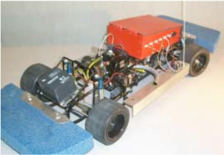
Figure 7: Radio Remote Control Car as a Vehicle Dynamics Test Bed
