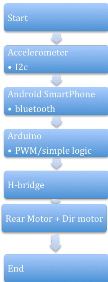
Figure 6: Process of Bluetooth Module Remote control using Android
