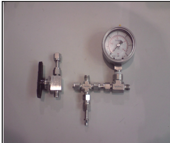
Picture 7: Valve and Pressure Gauge
