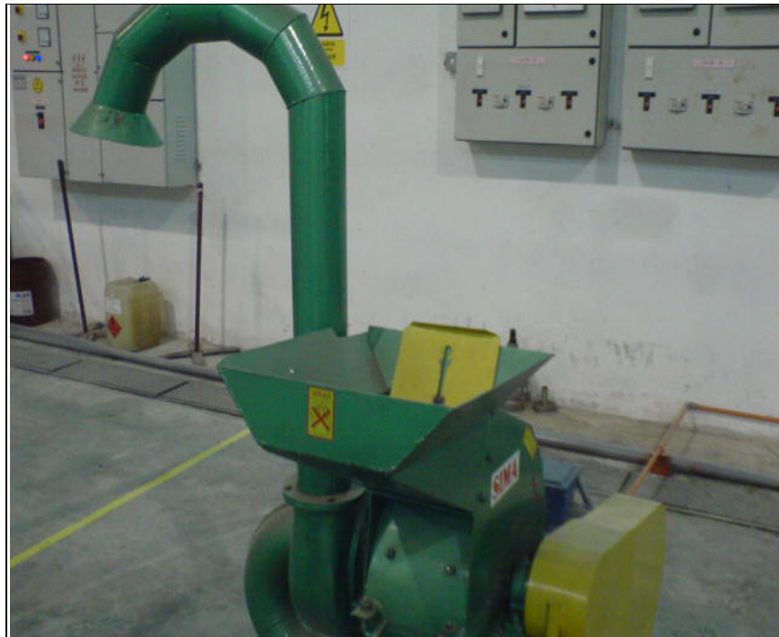
Figure 3.4: Grinder (SAMA Grinder model FG 400 x 200)
