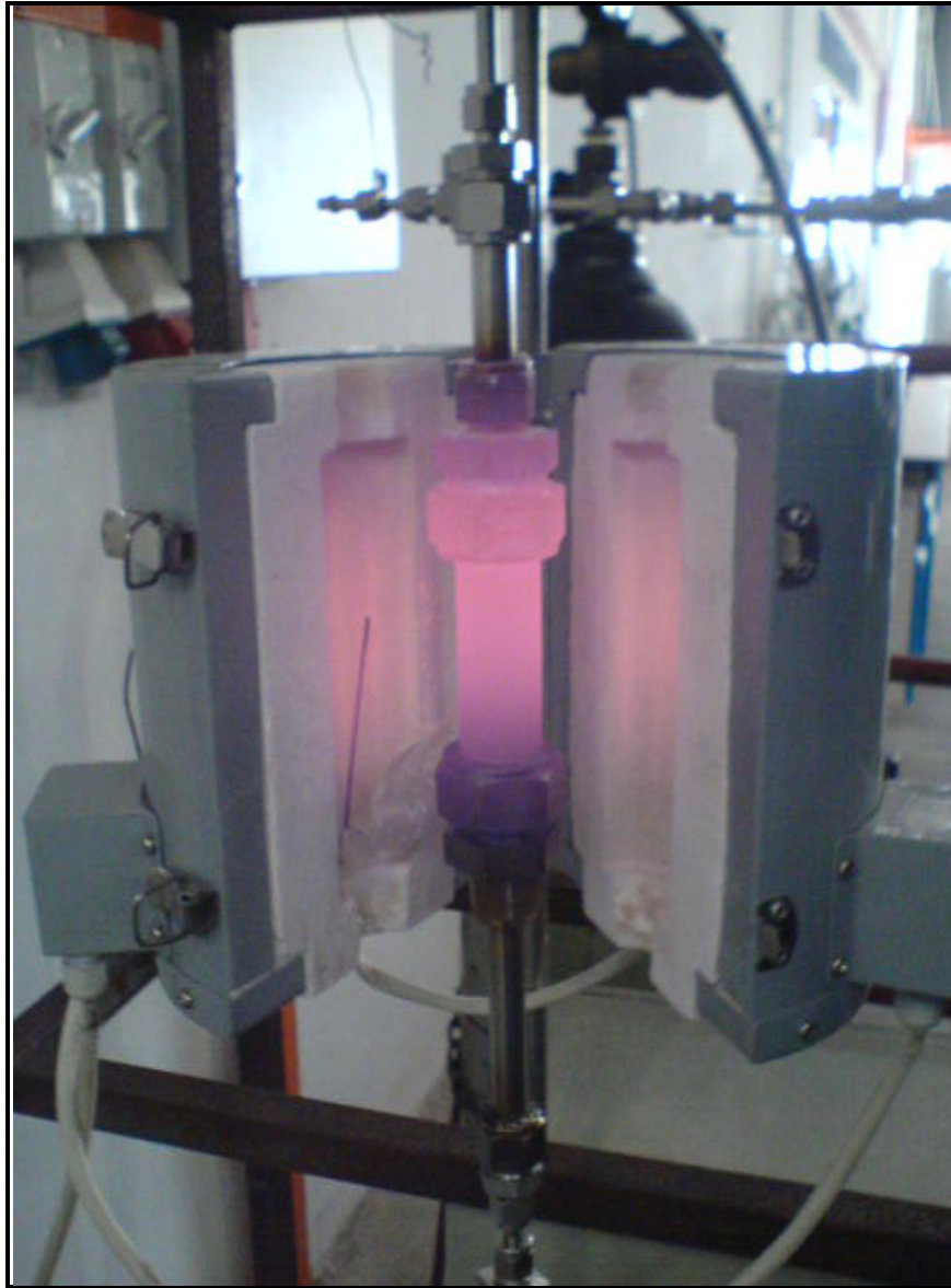
Figure 3.12: Reactor in Tubular Furnace
