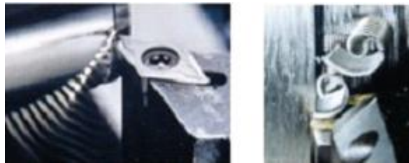
Figure17: Two major chip type, spiral and comma-shape chip. A small depth of cut produces spiral-shaped chips (left diagram) and longer depth of cut lead to comma-shape chips.
