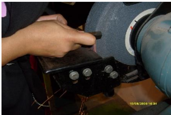
Figure 12: Hand holding the tool to “Break” the point saves resetting the angle on the tool rest.
