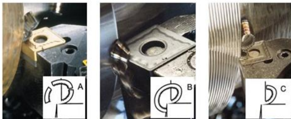
Figure20: There are three type of chip formation (A) self-breaking (B) breaking against the tool (C) breaking against the workpieces.
