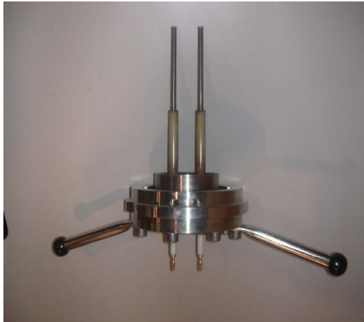
The Ignitor of Gas Fire Explosion. The place where the fuse is attached
