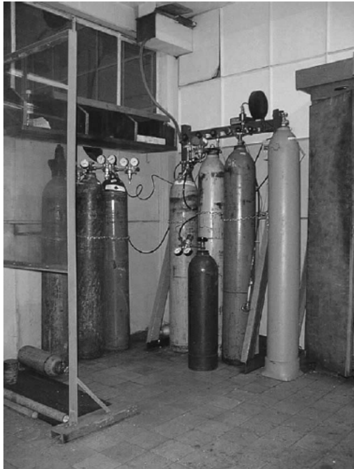
Figure 2.17: General view of the stand for precise preparing of the test mixtures.
