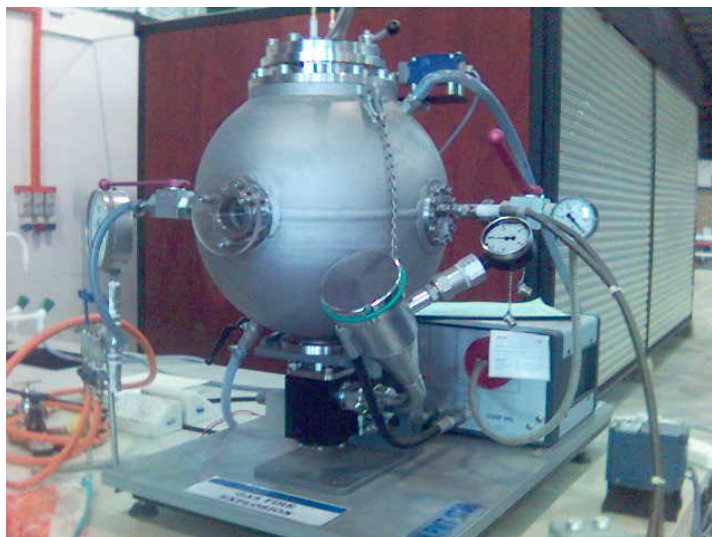
Figure 2.16: General view of 40 dm 3 explosion chamber.
