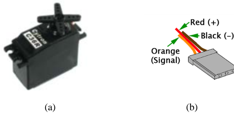
Figure 3.3 (a) C36R and (b) Wire Connection
