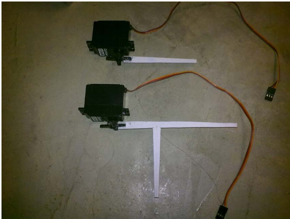
Figure 3.21: Actual Fin's Joint Structure
