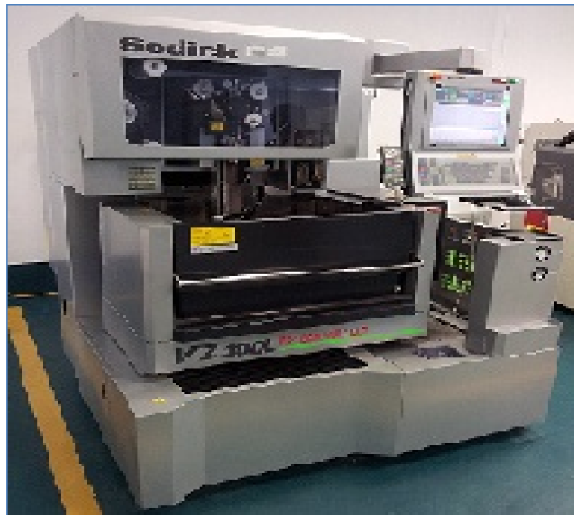
Figure 3.14: EDM wire cut
