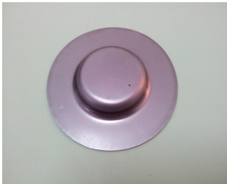
Figure 4.1: 10mm draw depth and 1mm thick of steel plate
