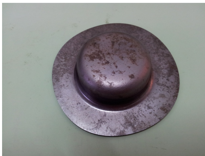
Figure 4.4: 20mm draw depth and 2mm thick of steel plate
