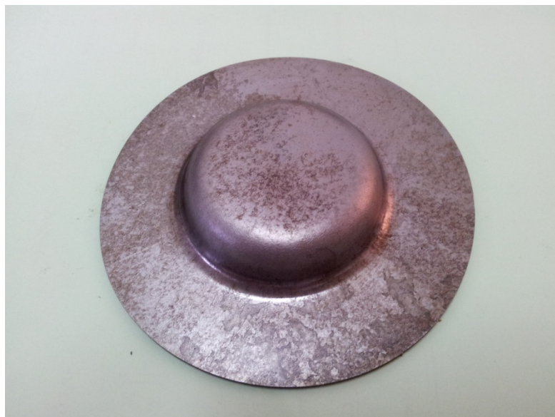
Figure 4.3: 10mm draw depth and 2mm thick of steel plate
