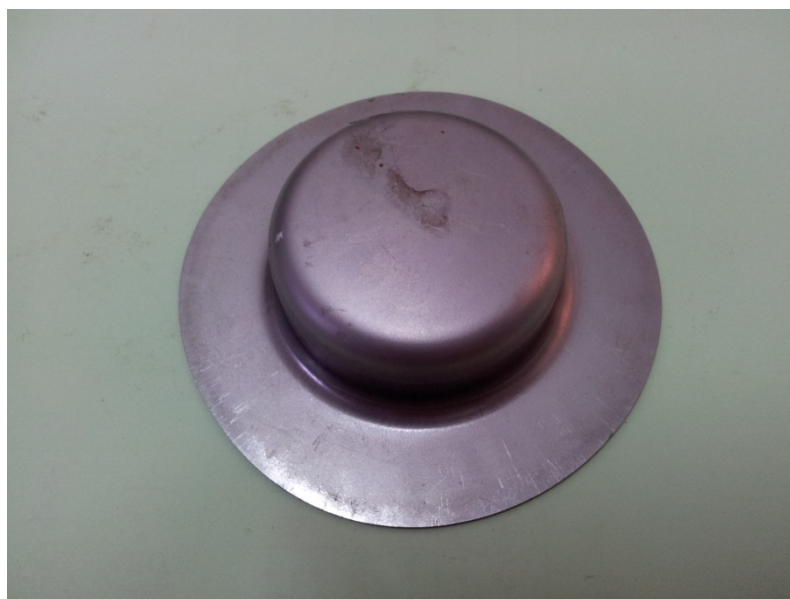
Figure 4.2: 20mm draw depth and 1mm thick of steel plate
