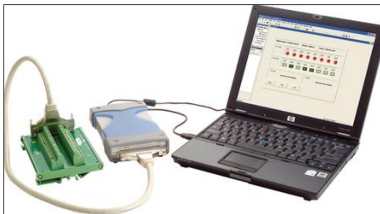
Figure 5.5: Interface instrument between U32352A, U2901A and PC [25]
