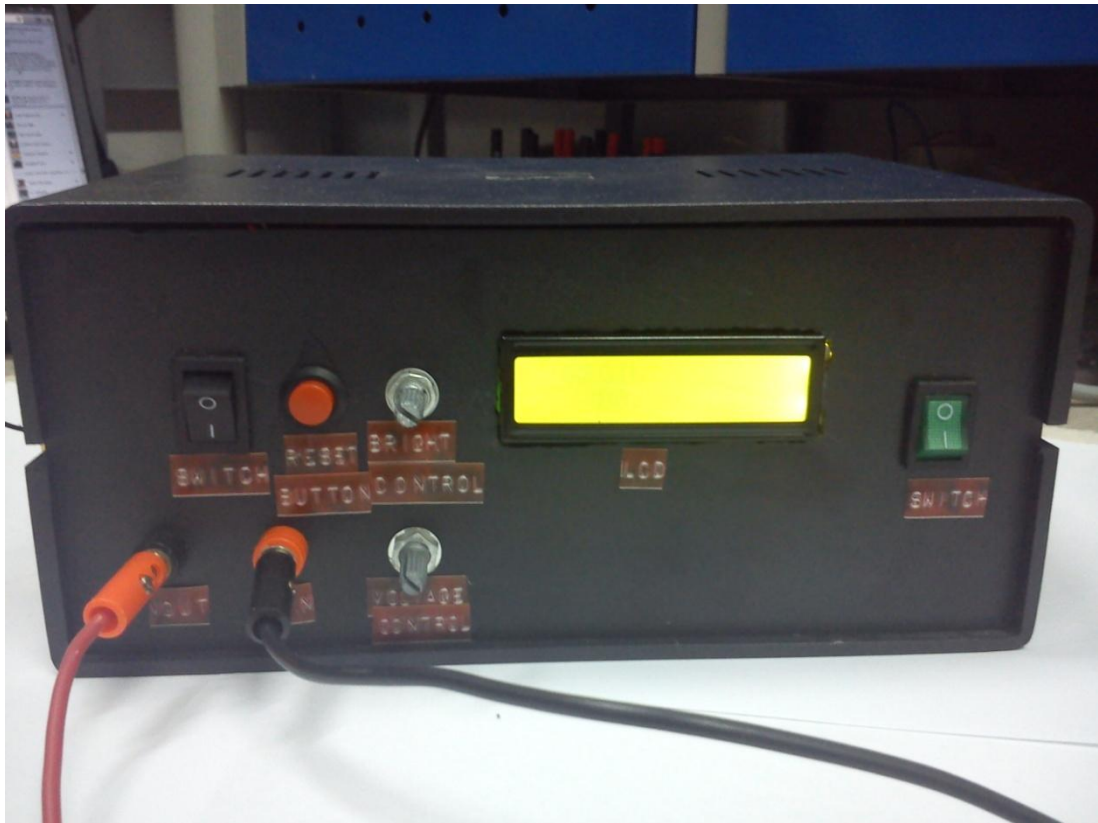
Figure 4.11 : Prototype Battery Impedance Tester
