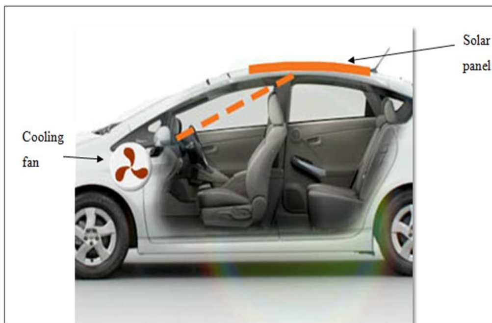
Figure 1.1: Model of a car using cooling fan to remove hot air out
