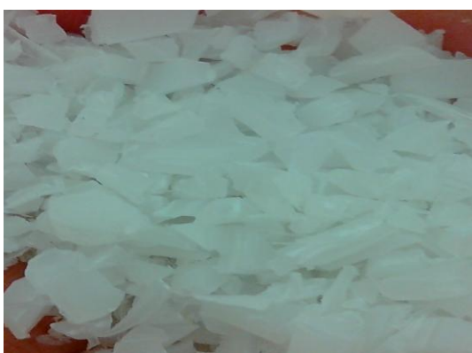
Figure 3.4: HDPE material that already been crushed through crushing machine and will be used as the recycled HDPE for this research.
