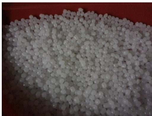
Figure 3.3: The virgin HDPE material supplied by Titan Chemicals Company.
